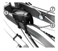
5. Place the spoke in the groove of the plastic piece, and tighten it slightly.
