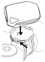
To detach the cycling computer from the bike mount, push the button and lift the cycling computer off the bike mount.
